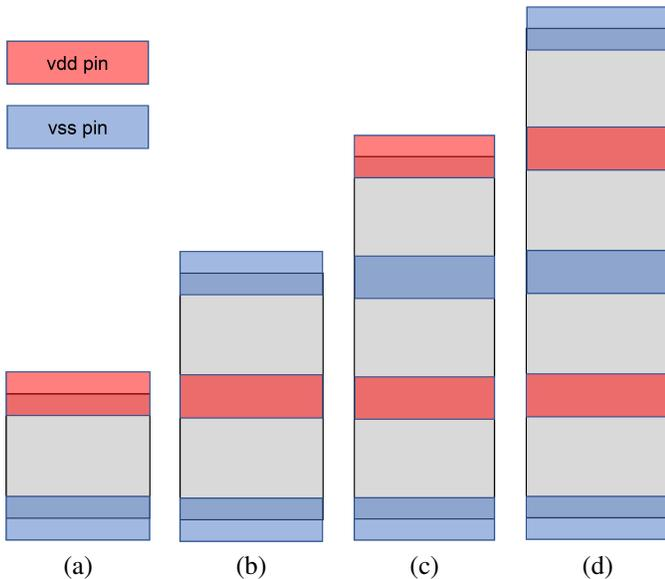
Fig. 1. Multi-deck cells with their *vss* and *vdd* pins. (a) a single row height cell; (b) a double row-height with two *vss* ports on top and bottom, and a *vss* pin in the middle; (c) a triple row height cells; and (d) a quadruple row height cell.
