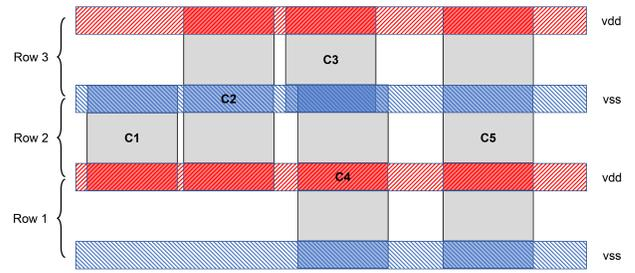
Fig. 2. An example showing multi-deck cells aligned with the P/G mesh defined in the design. *C1* and *C3* are single row height cells, *C2* and *C4* are double row height cells, and *C5* is a triple row height cell.
